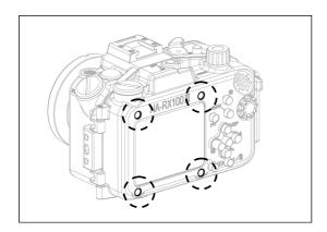
1. Remove the four rubber caps from the rear housing.
