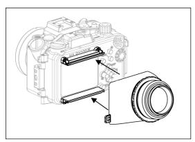
3. Attach the 25106 LCD Magnifier onto the rails above and below the LCD monitor window.
