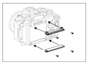
2. Attach the rails to the housing above and below the LCD monitor window as shown and fasten it by the screws provided.
